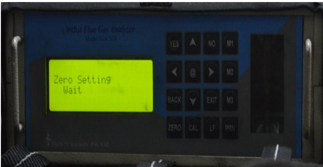
Fig 8.4: Caliberating the Gas Analyzer
