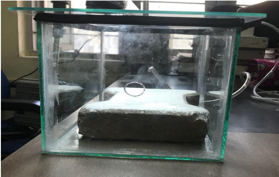
Fig 5.6: Glass chamber with a 2cm hole for insertion of Gas Analyzer probe
